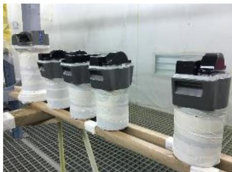
Coating of instruments with ClearSignal® biofouling control system is now underway at UVS workshops in Newcastle. Unlike anti-fouling systems that rely on active biocides and whose effectiveness degrades with time, ClearSignal® remains 100% effective for the intended life of the instrument.
